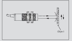
The light transmitter and receiver in a diffuse-reflection sensor are accommodated in one common enclosure. The light emitted from the transmitter is reflected diffused from the detected object. A part of this diffused reflection returns to the receiver and changes the switching status at the output when a certain intensity is exceeded. Accordingly, the texture and the colour of the object surface has a considerable influence on the object detection characteristics (presence – absence).
