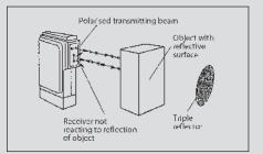
This is a special type of retro-reflective sensor. A special linear or circular polarised filter element (film) is placed between the transmit or receive elements and the glass light emitting face of the sensor.
