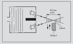
Convergent beam sensors, fixed focus The transmit and receive modules of convergent beam sensors are arranged at a defined angle to each other. The light cone of the transmitter and receiver are joined at a fixed focal point. This results in the active zone for the detection of objects being defined around this focal point.
