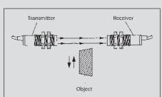
Through-beam sensors consist of an light transmitter (light source) and a spatially separated receiver. The light emitted by the transmitter is analysed by the receiver. An interruption in the light path, e.g. by an object, is evaluated and causes the output to switch.
