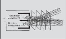
This is a special type of diffuse-reflection sensor. It is based on two receive modules or segmented receivers.
